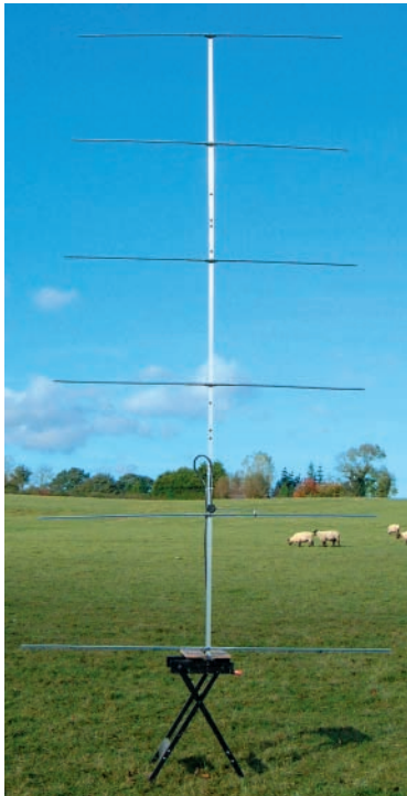
● Fig. 1: Pointing the whole antenna skywards by clamping it to a wooden workbench makes adjusting the matching arrangement fairly easy.
